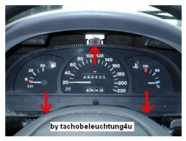
And last you have to unscrew these three screws therewith is speedo unit is free. Now pull out the speedo CAREFULY and disconnect the plug connectors behind it.
