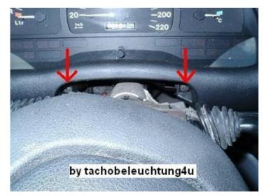
Now you have to unscrew these two screws and you can carefuly remove the cockpit covering.
