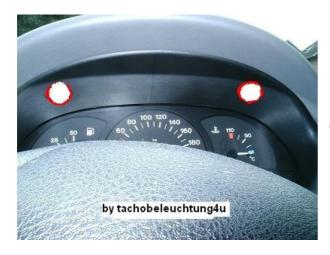
First you have to unscrew the two screws marked on the picture.
